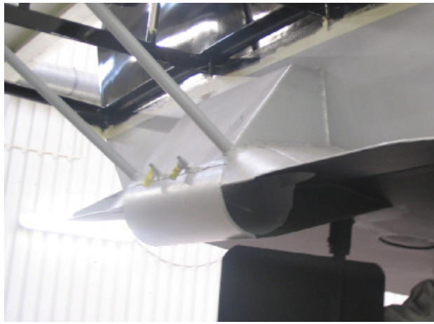
Professional subsequent fitting of stern thruster integrated into the hull.
