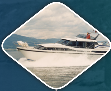
1984 The 115SX. Linssen's first steel semi-planing yacht, designed by Winfried H. Wilke.
